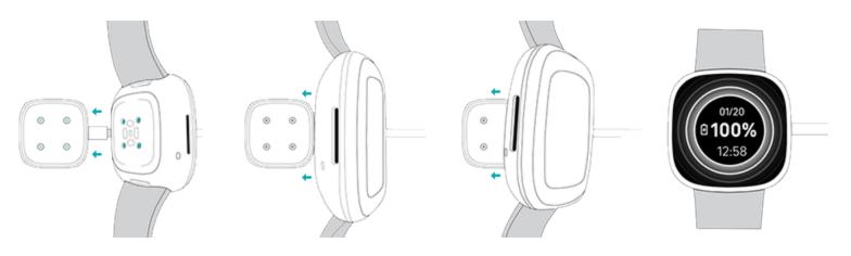
Charge Versa 3 for 12 minutes for 24 hours of battery life. While the watch charges, tap the screen twice or press the button to turn the screen on. The battery level appears for several seconds, then disappears so you can use your watch while it charges. Charging fully takes about 1-2 hours.
