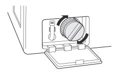
**8** Close the drain pump filter cover.
