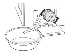
**5** Clean the pump filter and opening.
