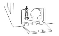
7 Insert the drain pump filter and twist it clockwise.
