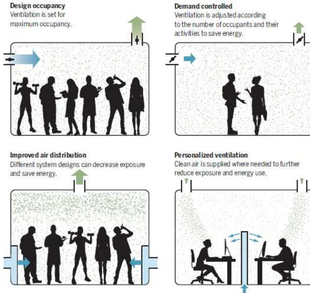
Flexible ventilation systems, dependent on the building's purpose. Ventilation airflow rates must be controlled by the number of occupants in the space and their activity.
